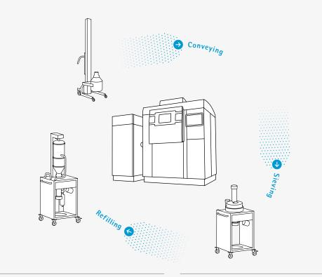
Material handling with the IPCM M extra modules enables the highest part quality and optimizes both productivity and economics. Together with the Comfort Powder Module, the risk of material contact is reduced to a minimum.
