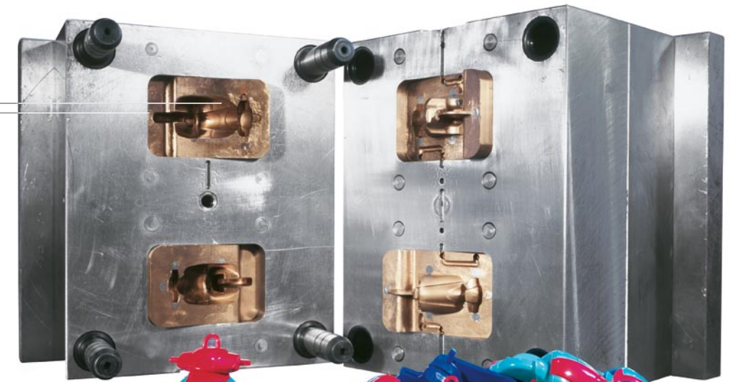
Twin coloured key ring, injection moulded with DirectTool.
