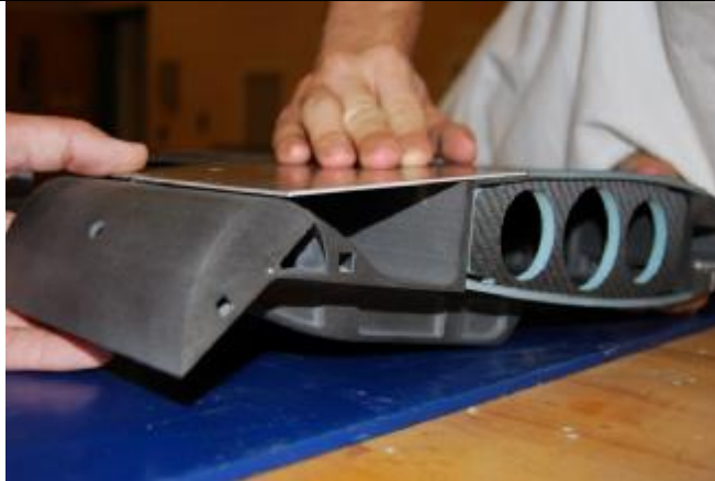
Trailing edge structure and flap of UAV wing, manufactured with plastics laser-sintering ( Courtesy Solid Concepts )
