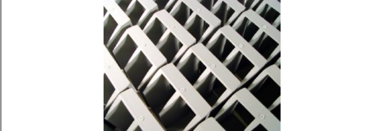
Shown above are control vanes for a Honeywell MAV (micro-air vehicle) made from Polyamide Nylon 12 in EOS laser-sintering equipment. There are four of these vanes per vehicle. (Photo courtesy Paramount PDS)
