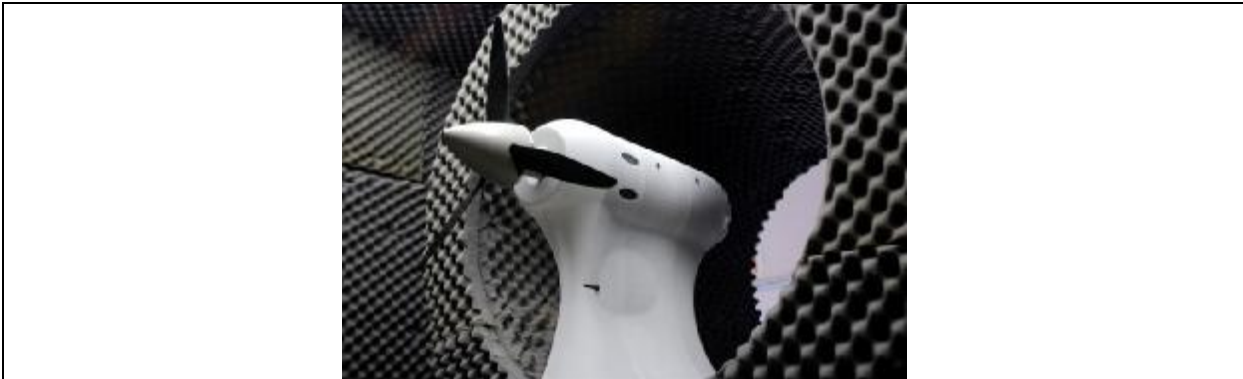
View of a UAV propeller dynamometer that features custom-designed laser-sintered shrouding. (Courtesy Northwest UAV)
