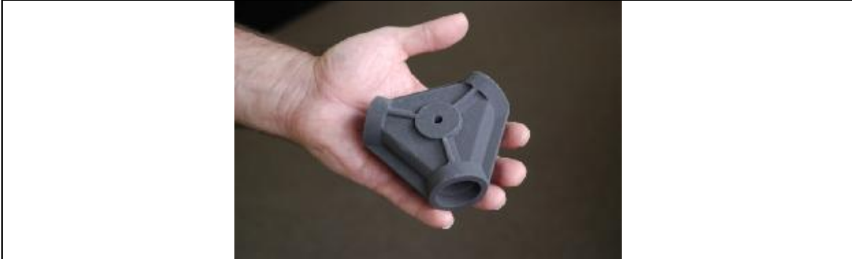
Shown is a laser-sintered polystyrene pattern used to make an aluminum casting for part of a three-blade, variable pitch propeller hub and blade assembly (Courtesy Northwest UAV)
