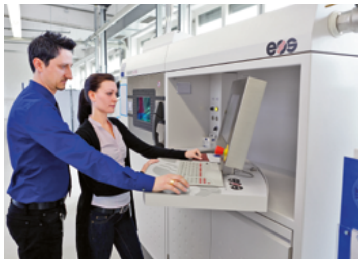
Manufacturing at MTU: One of the seven EOS systems that produces series components for engine construction (courtesy of MTU Aero Engines).
