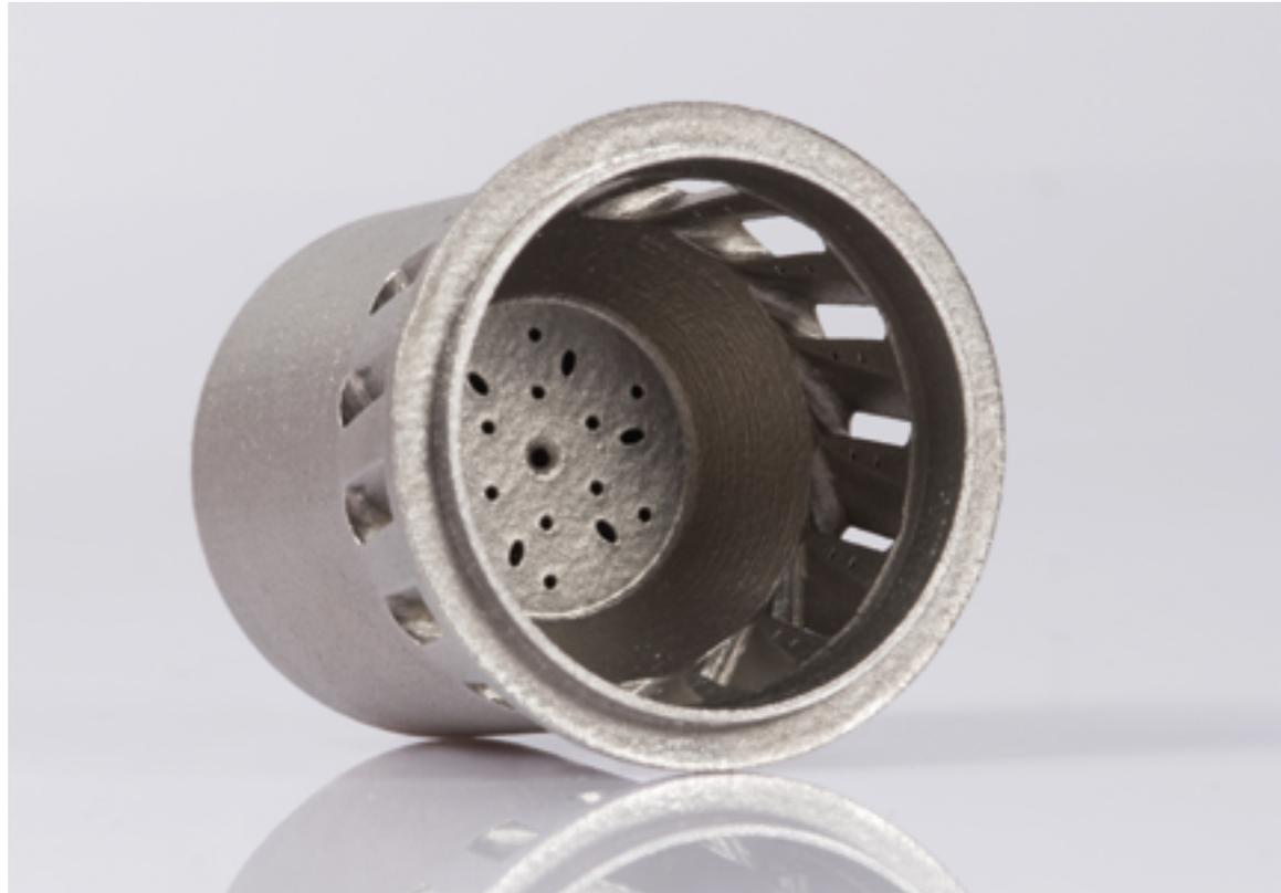
*Free choice of fuel: thanks to its complex channels, the burner produces a fuel / air mixture and can burn both gaseous and liquid fuels. (Source: EOS GmbH)*
