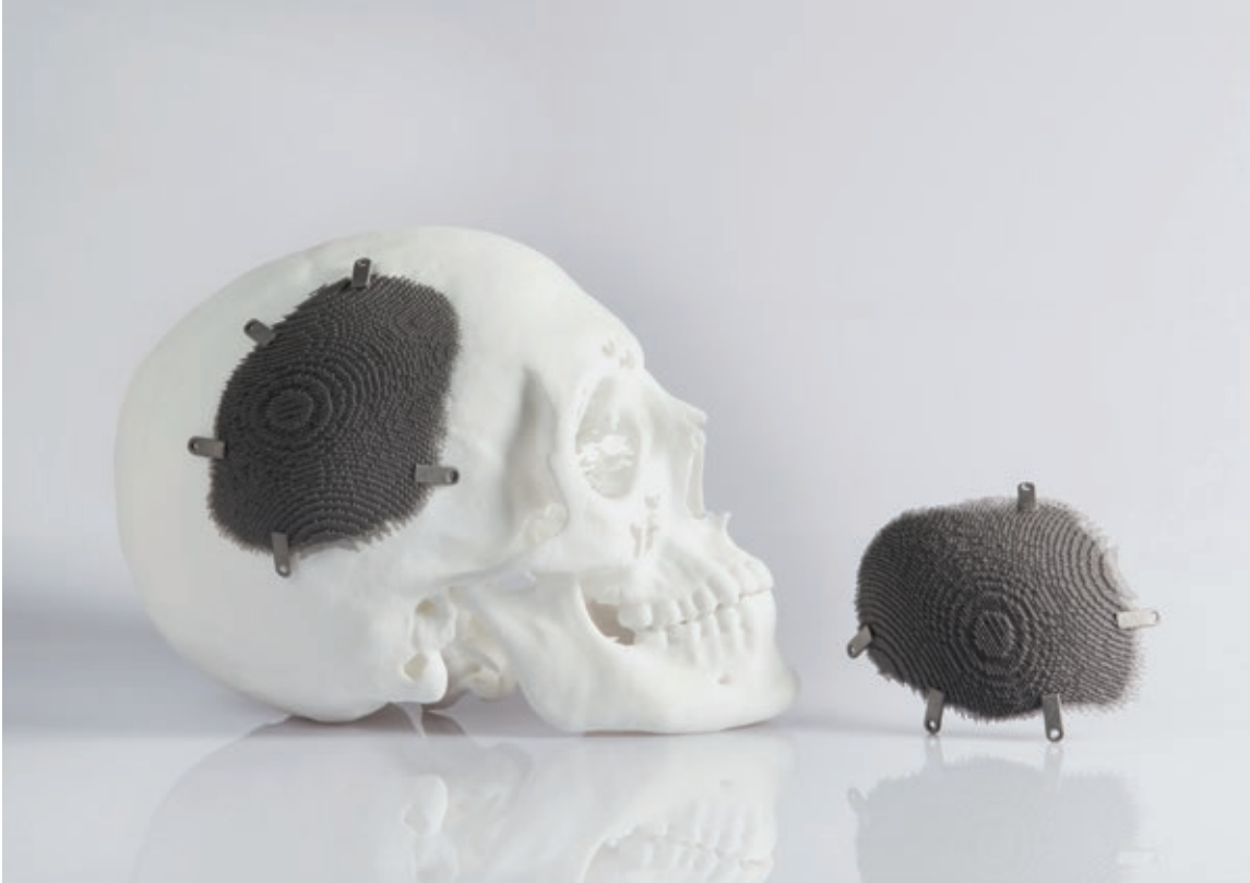
The porosity of the implant is 95%, so liquids can flow through with the least possible resistance and the bone tissue optimally coalesces with the outer edges (courtesy of EOS GmbH).
