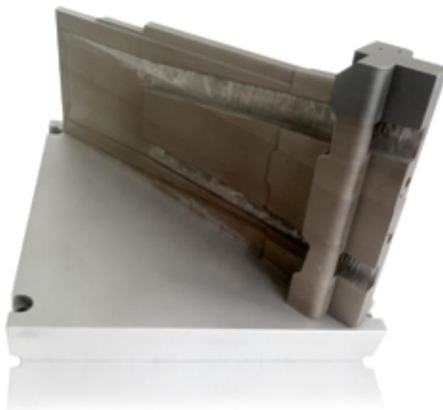
*Additive manufactured tooling insert on building platform: using EOS technology contributed to an extended maintenance interval and solved the problem of air humidity condensation and potential cavity corrosion completely (Source: Innomia).*
