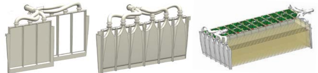
A complex battery system requires powerful heat dissipation – no big deal thanks to additive manufacturing (source: GreenTeam Uni Stuttgart)
