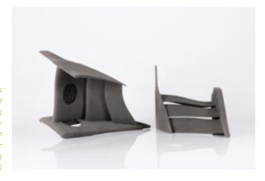
Optimized components thanks to perfected prototyping: Front wing cascade (on the left with internal lattice structure to save weight) of the Williams Martini Racing car. (source: EOS GmbH) materials are, as mentioned, difficult to work with, Williams Martini Racing has decided to additively manufacture prototypes for the wing to test the shape.
