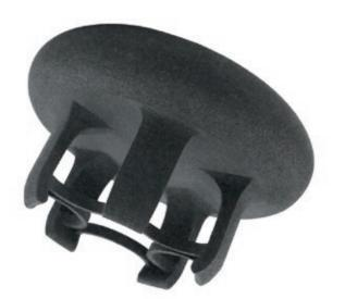
Integrated functions: when compressed air flows into a flexible membrane the claws of the gripper will open; likewise the system closes when the compressed air is turned off (Source: Kuhn-Stoff).
