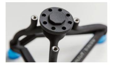
Customer-specific gripping system manufactured with an EOS P 396. (Source: trinckle)
