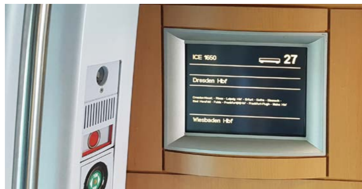
Monitors in the interior of each ICE train display information about the speed, time of day, and upcoming station to passengers. (Source: Hasenauer & Hesser)
