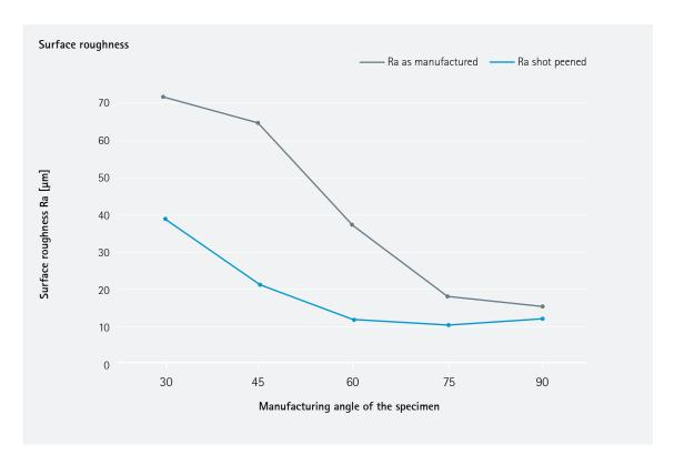
The surface quality was characterized by optical profiling from downfacing surfaces according to internal procedure. The 90 degree angle corresponds to vertical surface.
