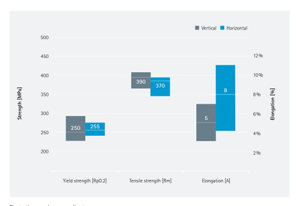
The testing was done according to EN 2002-001 2005 on round specimen machined according to standard Annex C. Results of both horizontal and vertical building direction are presented.
