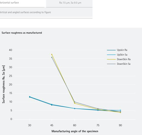
The surface quality was characterized by optical measurement method according to internal procedure. The 90 degree angle corresponds to vertical surface.
