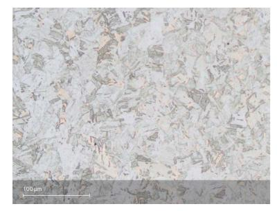
Heat treated microstructure. Etching; ASTM E407-94
