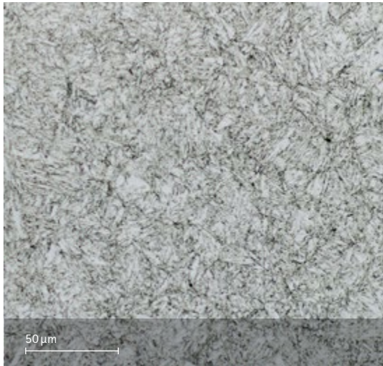
Micrograph etched, heat treated state Etchant: Oxalic acid
