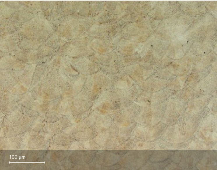
As manufactured microstructure. Etchant: Kalling's II
