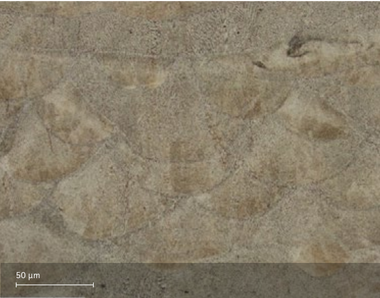
As manufactured microstructure. Etchant: Kalling's II
