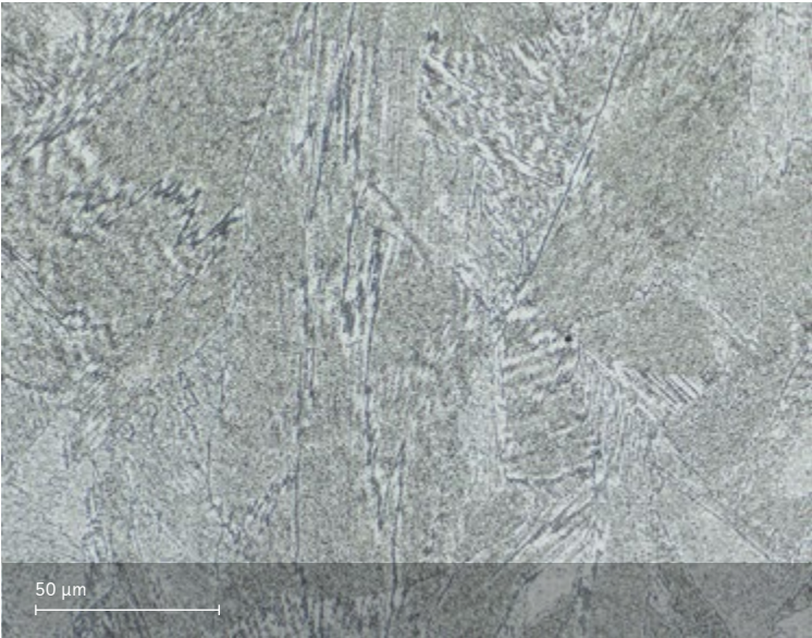
Heat treated microstructure. Etched according to ASTM E407-07.
