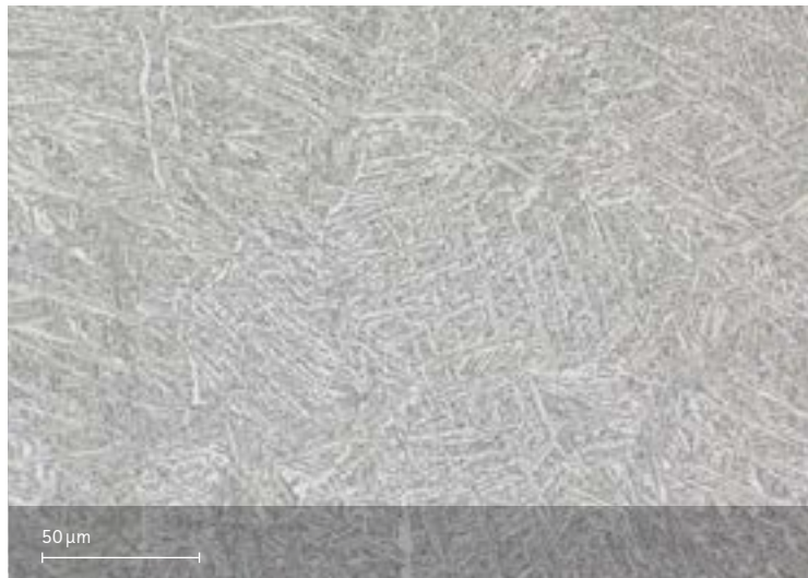
Heat treated microstructure. Etched according to ASTM E407 modified recipe #190.
