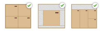
The parts must be arranged within the load carrier so that the weight is evenly distributed. Sensitive parts must be properly padded.
